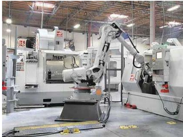
Fig. 15 - one Robot can manage many CNC machines
