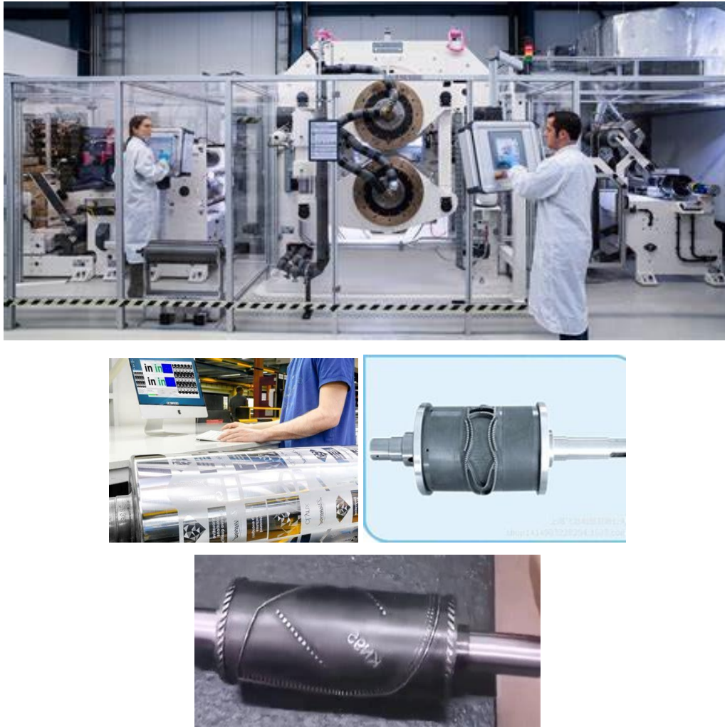
Fig.10 – cutting roller of hygiene products for mask converting
